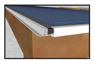
10. Once the sheets are in place use the HawK top cap which should click firmly into place. For the end sheets add the additional end bar infill.
