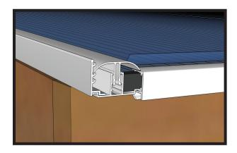
11. Line up the hole of the endcap with the screw port on the pvc top cap and screw into position.
