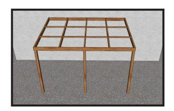
2. Line up and cut the bars and edge bar fills so that they are the same length as the framework rafters with an additional 50mm overhang.
