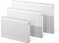
Internally welded with a final coating of white enamel (RAL9016) each radiator is degreased and zinc phosphated before being coated with waterbased cathophoratic paint. The final coat is applied using an epoxy polyester electrostatic powder coating system that is baked to a hard finish. You also have the protection of our 'Kartell No Quibble Guarantee' against faulty manufacture which lasts for 10 years. All radiators come complete with factory fitted top grille and side panels.
