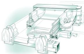
**YORK Bars for 16, 25 & 35mm polycarbonate sheets on spans of up to 4M.**
