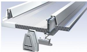
Designed for mono-pitched roofs, **YORK** glazing bars are available in two grades – The system 7 bar will carry 16, 25 and 40mm polycarbonate roof sheets up to spans of 3 metres, whilst the heavier gauge System 8 bar will carry 25mm and 35mm polycarbonate roof sheets up to spans of 4 metres. Designed to be quick to install with fewer components needed for each bar.
