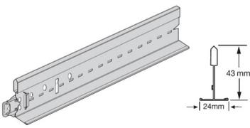
The white-faced, galvanised, steel interlocking frame is fast and easy to install. An angle section is fitted around the walls, then the main 'T' sections rest on these and reach across the room. The spacer 'T's are then fitted to create the desired tile space.
