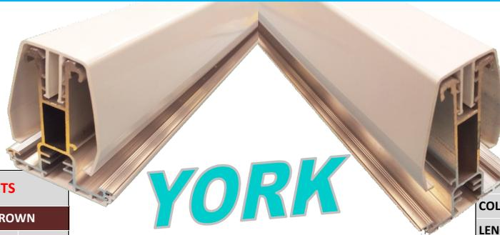
The **System 8** glazing bar has a 80mm high aluminium core and is the more robust version with spans up to a maximum of 4M without support and comes with the option of a 6M bar.
