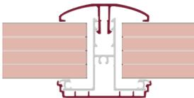
The **EDEN & HAWK** bars must have structural support under their entire length, whilst the **AVON** with stronger aluminium core can span across purlins that are no greater than 600mm (approx. 2ft) apart. This makes them ideal as a replacement to corrugated roofs as the structure should not need changing if originally built correct and in good order.
