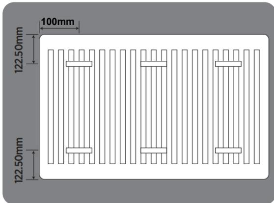
**INSTALLATION** A minimum of 100mm from the floor bottom of the radiator is required. There are two options for the valve centre to wall dimension which is dependant on how the wall plate is fitted. Type 11—40mm or 55mm, Type 21—65mm or 80mm, Type 22—82.5mm or 97.5mm
