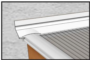
$14^{\text{FIX PVC}}$  flashing to wall and cut appropriately to sit across canopy.
