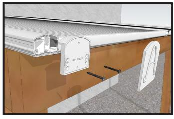
$12^{\mbox{\scriptsize finally fix}}$  the bar endcap  $13^{\mbox{\scriptsize click}}$  the face covering into place with 2 screws.
