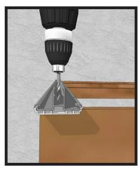
4 FIX THE CONNECTED ALUMINIUM BAR AND BASE TO THE CENTRE OF EACH RAFTER. DRILL AND FIX ALONG THE RAFTER AT APPROXIMATELY 600 CENTRES.
