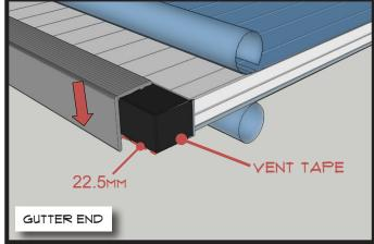
THE SHEET ENCLOSURES SHOULD BE CUT TO SHEET WIDTH - 45MM LENGTHS AND POSITIONED OVER THE TAPES CENTRALLY.
