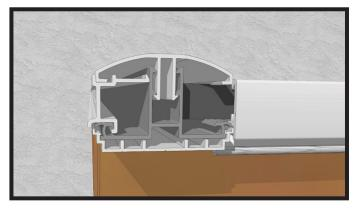
11 FOR THE TWO BARS AT EACH END, PLACE THE BAR INFILL INTO PLACE BEFORE ADDING THE TOP CAP. THE TOP-CAP SHOULD HOLD THE INFILL FIRMLY IN PLACE.
