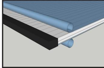
THE PROTECTIVE FILM ON THE SHEETS SHOULD BE PEELED BACK APPROXIMATELY 50MM ON ALL EDGES AND ON BOTH SIDES. ENSURING THE SHEET IS FREE FROM DUST MOISTURE AND ANY OTHER DEBRIS THE SHEET TAPES SHOULD BE APPLIED TO THE TWO SHEET ENDS. VENT TAPE FOR THE GUTTER END AND AND ALL TAPE FOR THE WALL END.
