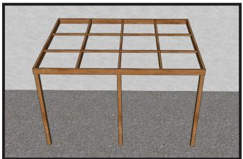
1 CONSTRUCT SUITABLE FRAMEWORK. THE RAFTERS UPON WHICH THE BARS WILL SIT SHOULD BE POSITIONED AT 'WIDTH OF SHEET + 20MM' CENTRES. SO IF YOU'RE USING 1045MM WIDE SHEETING, POSITION THE RAFTERS AT 1065MM CENTRES.
