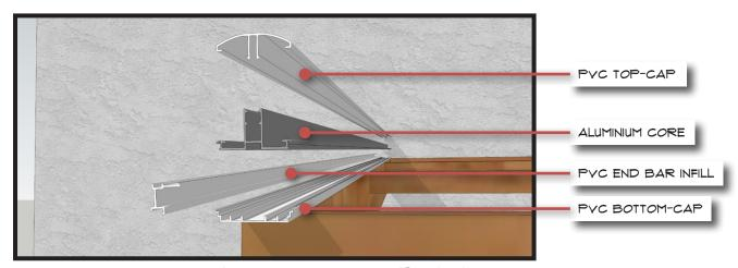
2 DIAGRAM SHOWING HOW THE COMPONENTS FIT TOGETHER TO FORM A TYPICAL AVON BAR. THESE PARTS SHOULD BE CUT TO THE SAME LENGTH AS THE RAFTERS WITH AN ADDITIONAL OVERHANG OF 60MM
