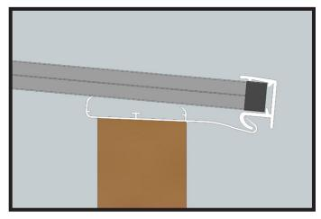
9 POSITION THE SHEETS INTO PLACE. THE BOTTOM LIP OF THE SHEET ENCLOSURE SHOULD TUCK IN TO THE EAVES RETAINER WHICH WILL HELP HOLD THE SHEET IN PLACE.
